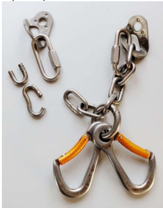
Photo 1: The FIXE anchor, where 2 links are broken.
